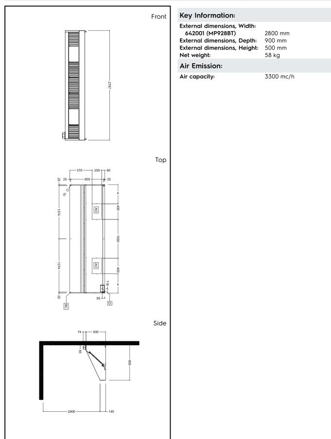
Ventilation Equipment 430 S/S Wall Hood+Filters 2800X900mm
